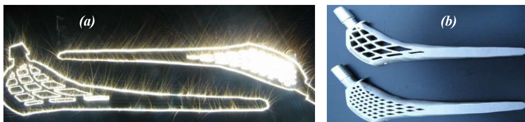
Figure 1: (a) 3D additive manufacturing (b) The manufactured endoprostheses
