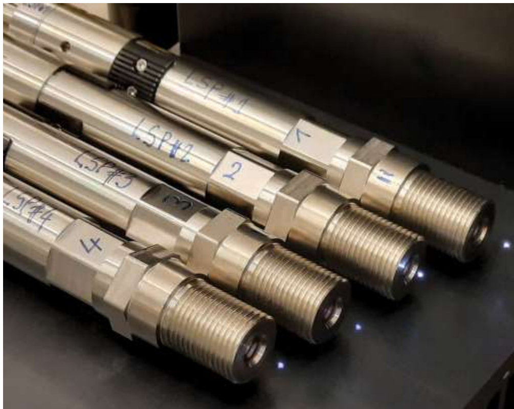
Figure 2. A set of four laser spark plugs during assembling and performance tests. The small sparks are laser plasmas, created due to air breakdown.
